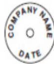
External Groundline Treatment Contractor shall install on poles that have been bored, sounded, and externally treated in accordance with SCE Specifications.
