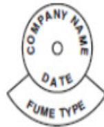
Fumigant Treatment Contractor shall install on poles that have been internally treated with fumigants in accordance with SCE Specifications.
