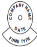
Fumigant Treatment Contractor shall install on poles that have been internally treated with fumigants in accordance with SCE Specifications.
