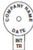
External Groundline Treatment plus Internally Treated with a Preservative Solution. Contractor shall install on poles that have been bored, sounded and externally treated as well as internally treated with a preservative solution in accordance with SCE Specifications.
